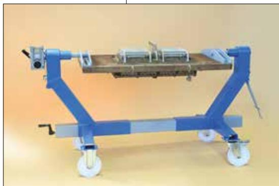
*The machine is designed to be both easy to use and completely safe for the operator, who only needs to perform two basic operations: install the die and fix it to the dedicated support, then adjust its position using a crank to attain the most suitable position for maintenance.*
