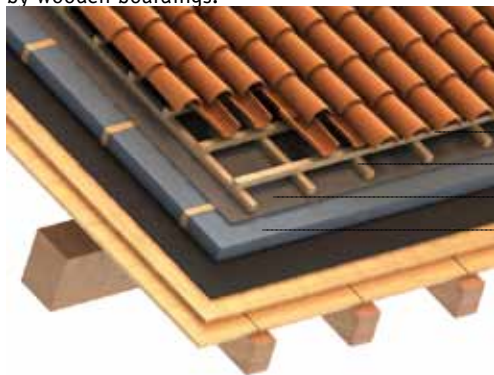
Figure 2 – Undermantle ventilation through single cavity.
